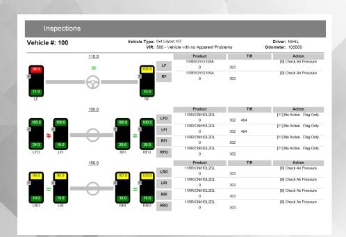
The Vehicle Inspection Report shows a footprint of the vehicle and instantly color coordinates the tires based on fleet parameters.
