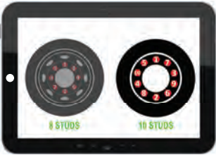
Define stud profile and torque
